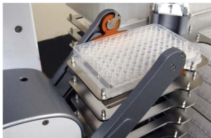
Figure 8: BenchCel robot picking up microplate from the Agilent Labware MiniHub.
