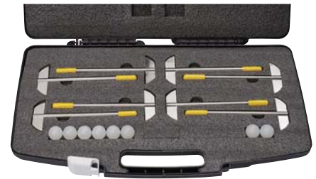
Paddles in storage case (included), 6/pk (p/n 16-3602). Six paddles are included in the kit, although the case will store eight.
