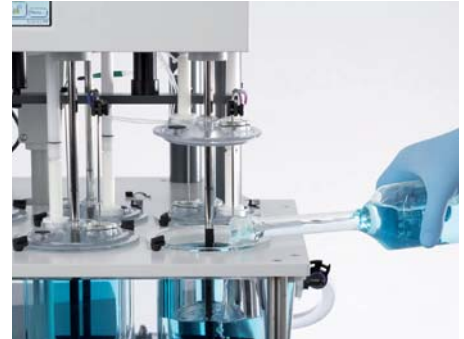
Hands-free evaporation cover suspension supports easy media addition.
