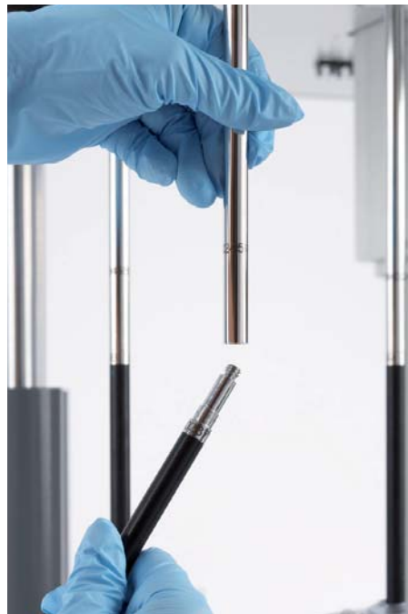
Upper shaft receptor and lower interchangeable paddle piece.
