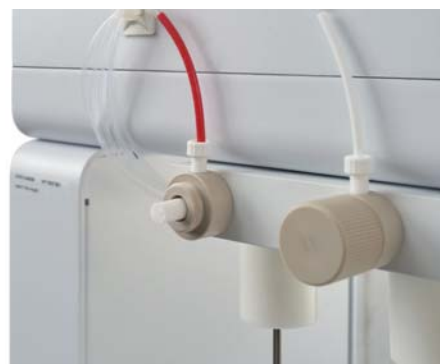
In-line filter housing (PEEK) (p/n K1200-00855), shown on optional mounting bracket.
