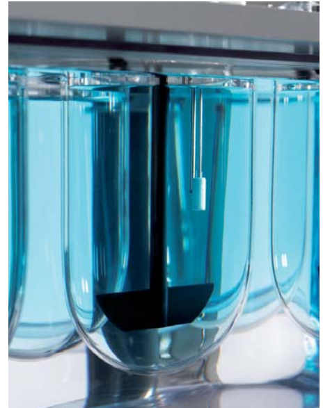
Non-resident sampling cannulas in a TruAlign vessel on the 708-DS.
