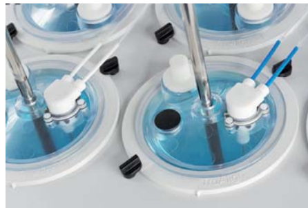
Resident cannula kit on the 708-DS. See table below for available kits.
