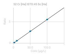
Calibrations for low level trace elements, using helium mode.
