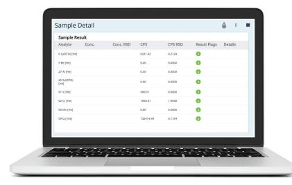
Color-coded flags save time when checking run status and QC results. The method will be customized to include your desired actions in the event of a QC failure e.g. recalibrate and rerun if the result is within a specified limit.
