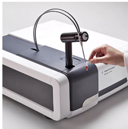
The Cary 60 UV-Vis Spectrophotometer with fiber optic accessory
