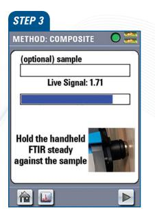
During sampling, the progress bar shows the advancement of the data collection.
