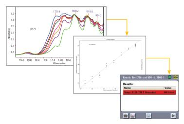
Composite thermal damage is represented in the MicroLab Mobile software. Behind the simple-to-use results screen, powerful calibrations embedded in the software provide a method specific to the analysis parameters. The result is color coded in red to show that the sample exceeds the critical threshold, indicating thermal damage.
