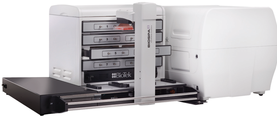
BioSpa 8 transfers microplates from its incubator to Cytation.
