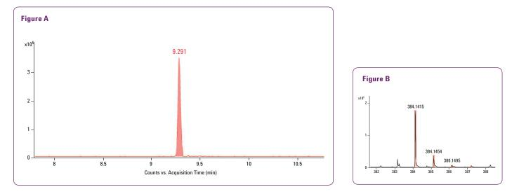
**For pesticide analysis, the 6550 iFunnel Q-TOF demonstrated** (Figure A) 10-fold sensitivity gain for a poor responding pesticide (fluazifop-butyl) in pepper matrix. Extracted ion chromatogram shows excellent detection (S/N 1200) on 10 ppb fluazifop-butyl and (Figure B) confident compound identification of fluazifop-butyl with an excellent library match score of 98 based on a mass error of only 0.5 ppm and correct fit of isotope abundance and spacing.
