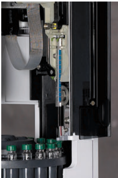
Blue line autosampler syringe shown in 7693A ALS, G4513-80204
