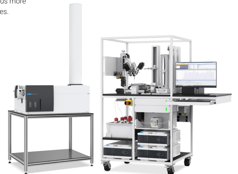
The RapidFire 400 can be connected to TOF, Q-TOF, or triple quadrupole MS.
