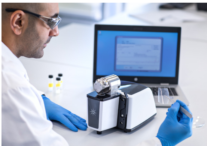
Figure 3. The DialPath accessory can be used to measure polymer films.
