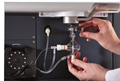
Multimode Sample Introduction System (MSIS)
