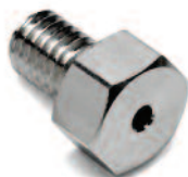
Stainless steel male nut, 1.6 MN, for 1/16 in tubing, 8001-0805
