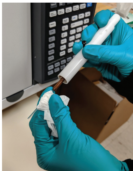
Figure 30. Using a lint-free wipe to clean the sides of a glass probe after adding sample to lower the possibility of carryover.
