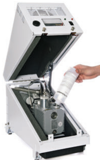
Quiet Cover GC/MS, with open-access cover
