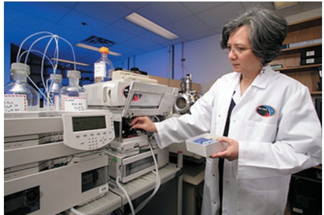
An NRC researcher uses a liquid chromatography-mass spectrometry system to quantify toxins in shellfish samples.
