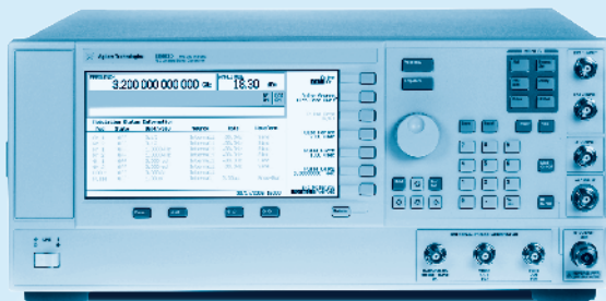
Option UNY for the PSG Series signal generators, including the E8663D shown here, provides outstanding close-in and pedestal phase noise for the most demanding applications
